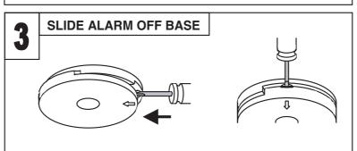
WITH THE SCREWDRIVER STILL INSERTED, PUSH THE LOWER HALF OF THE ALARM AWAY FROM THE SCREWDRIVER, IN THE DIRECTION OF THE ARROW ON THE COVER
